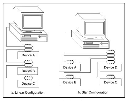
Figure 1-1. Linear and Star System Configuration
