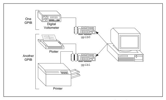
**Figure 1-2.** Example of Multiboard System Configuration
